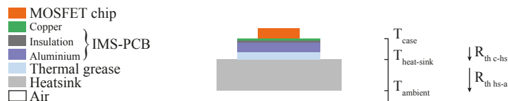
Fig. 5.7 Sketch of the thermal interface between the chip and the ambient for a Insulated Metal Substrate (IMS) based Printed Circuit Board (PCB) mounted MOSFET. Because of the time constants of the system, only the steady-state regime is taken into account.
